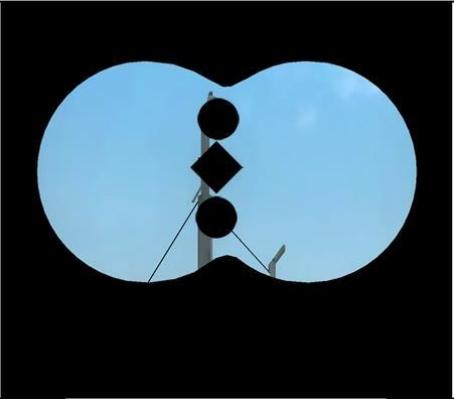
The image shows a signal for a self-propelled dredging machine. It consists of a vertical mast with two black circles, one above the other, and a black diamond shape between them. The signal is viewed through a blue, oval-shaped lens against a black background. | <ul style="list-style-type: none"><li>• <b>Самоходный дноуглубительный снаряд с волочащимся грунтоподъемником на ходу</b></li></ul> |
