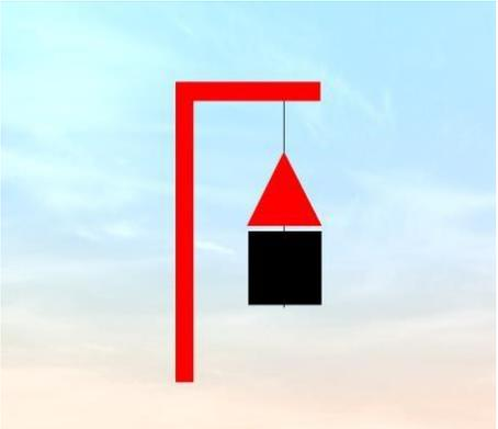
The image shows a semaphore signal against a blue sky background. A red T-shaped arm is positioned vertically. A red triangle is suspended from the top horizontal bar, and a black square is suspended from the vertical stem below the triangle.                                                            | <ul style="list-style-type: none"><li>• <b>Ход закрыт для движения сверху</b></li></ul> |
