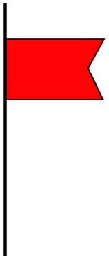
The image shows a signal for a vessel carrying dangerous cargo. It consists of a vertical black mast with a red pennant flag attached to the top.                                                                                                                    | <ul style="list-style-type: none"><li>• <b>Судно с опасными грузами</b></li></ul>                                                   |
