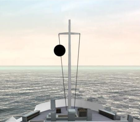
A photograph showing the mast of a ship at sea. A black ball is suspended from the mast, which is a signal for a vessel at anchor. | <ul style="list-style-type: none"><li>• Судно, стоящее на якоре</li></ul>                        |
